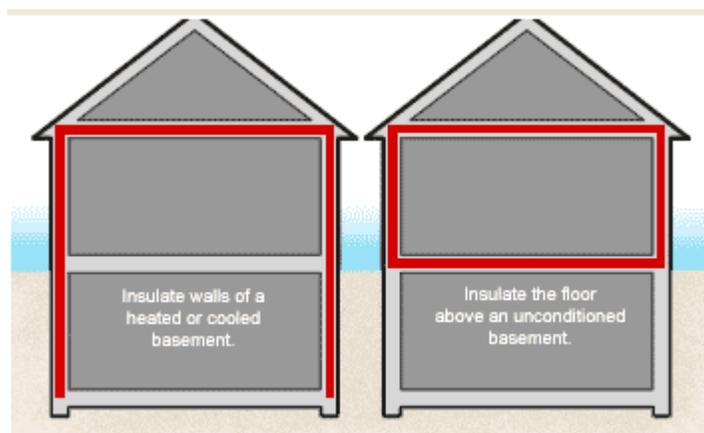
Walk-outs and slab-on-grade need the slab insulated by one of the methods shown below:
